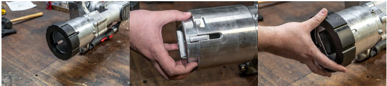
Figure 4: Installing the guide collar in a PGD4000X-DOT
