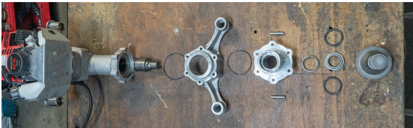
Figure 8: View when lower driver body is removed
