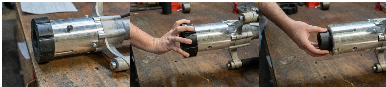
Figure 2: Installing the adapter sleeve on a PGD4000X-PFR
